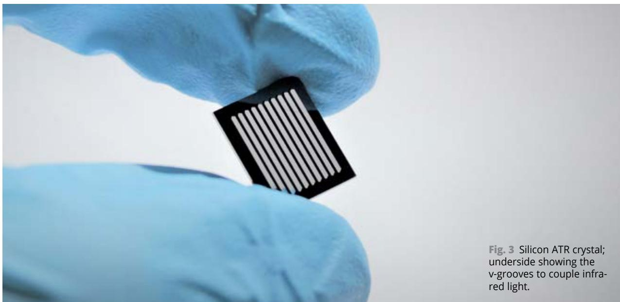
**Fig. 3** Silicon ATR crystal; underside showing the v-grooves to couple infrared light.
