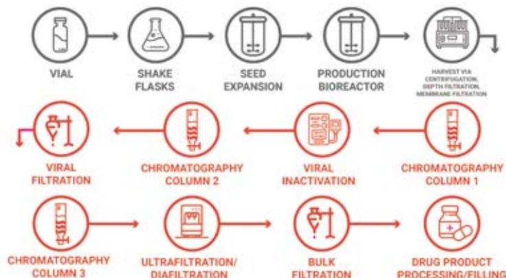
**Fig. 2** The overall biopharmaceutical process, both upstream (grey) and downstream (orange); from cell isolation to the production of the biopharmaceutical. (Adapted from [10])
